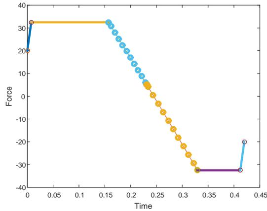
FIGURE 13. Driving force  $u$  for the case 4 with  $tff = 0.42$ ,  $xf = 0.1$
